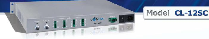
The rack-mountable CL-12SC fiberoptic baseband video multiplexer is ideal for transmitting 1 channel of baseband video, 1 channel of an RF Audio Subcarrier (4.5 MHz) and up to 4 channels of baseband audio on one fiberoptic cable. The CL-12SC operates by digitizing and multiplexing video, audio subcarrier and audio onto a high-speed serial cable.
